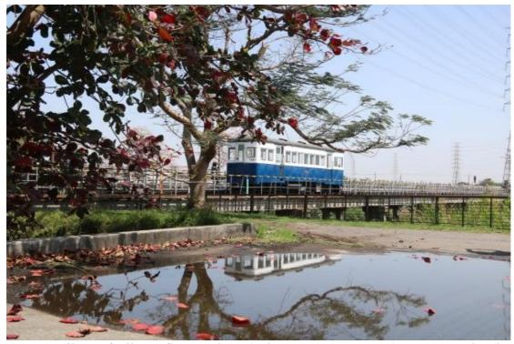
No 524 rail car of Xihu Refinery Taisuco(Taiwan Sugar Company) was restored and came back to run in last December. This is one of typical type of rail cars of Taisuco. It was modified in 1950s' from a originally passenger car made in 1949 and was retired in 1980. It had a unique feature of its power transmission and regulate systems similar to those of buses or trucks by mechanical transmission and clutch.
